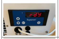
1. The toilet should be in standby mode (rdY) and no messages in addition to SEr1 should be displayed.
