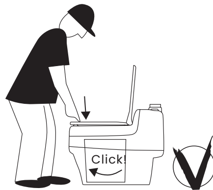
Make sure that the waste bucket rotates by pressing the seat down.
